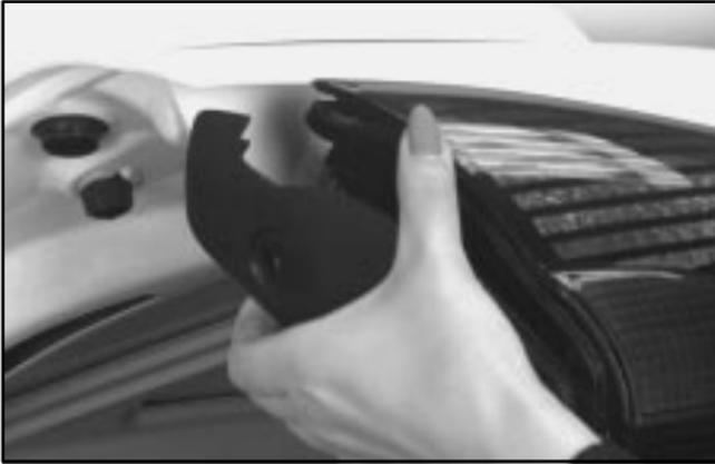
4. Lift up on both plastic side flaps at the same time (driver's side shown) and lift the assembly out.
