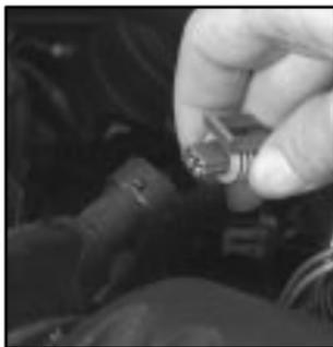
3. Disconnect the electrical connector which is attached to the air temperature sensor located in the hose. This will allow you to lift the rear portion of the air cleaner.
