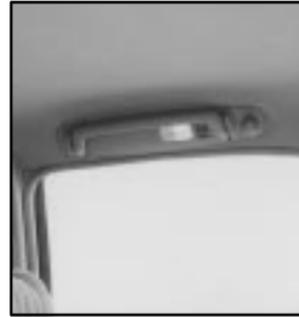
These overhead lamps and the interior courtesy lamps will come on when you open the doors.
