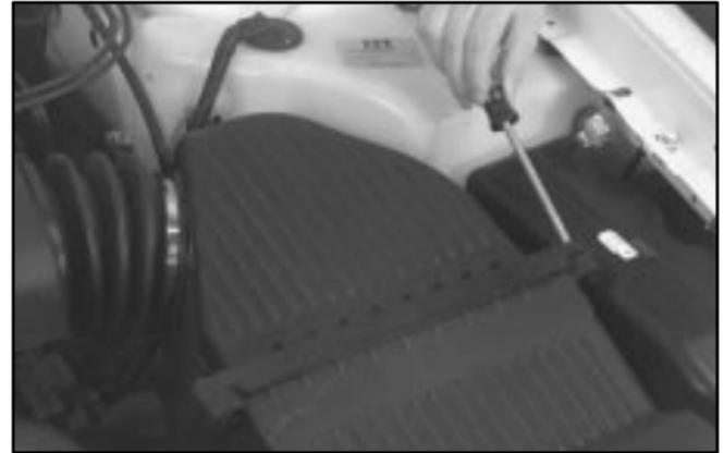
1. Remove the screws on the air cleaner housing cover.
