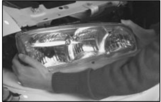
2. Slide the headlamp assembly outward (to the left) and lift it out.
