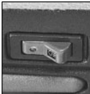
The fog lamps switch is in the front of the front reading lamps.
