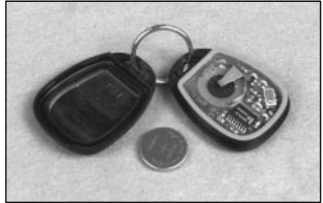
For battery replacement, use one Duracell® battery, type DL-2032, or a similar type.
