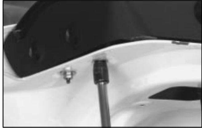
3. Remove the five nuts that hold the assembly in place with a 10 mm socket. Pull the carpet up and out of the way to remove the center nut. (There are two nuts on the driver's side, two on the passenger's side and one in the middle.)
