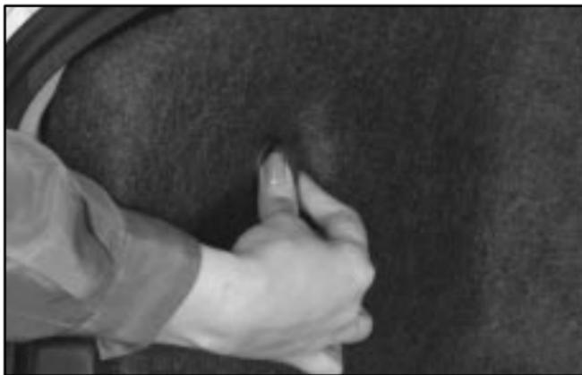
1. Remove the plastic nut holding the carpeting in place.
