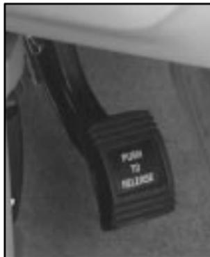
Your vehicle has a PUSH TO RELEASE parking brake. To set the parking brake, hold the regular brake pedal down with your right foot. Push down the parking brake pedal with your left foot. If the ignition is on, the brake system warning light will come on and a single chime will be heard.
