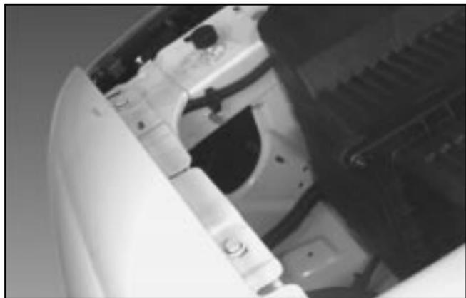
1. Reach behind the headlamp assembly and turn the bulb assembly counterclockwise to remove the bulb assembly.
