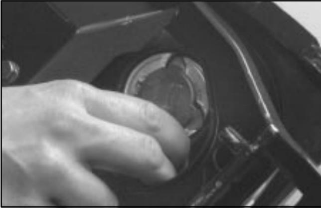
3. Tip the assembly and turn the bulb assembly counterclockwise to remove it.
