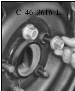
9. Replace the wheel nuts with rounded end of the nuts toward the wheel.
