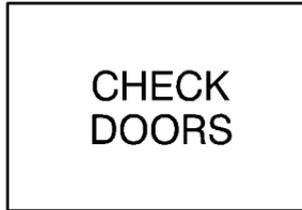
This light is part of the Systems Monitor. This message means that either the driver's door or one of the passenger's doors is not completely closed.
