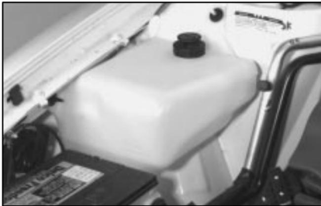
The vehicle must be on a level surface. When your engine is cold, the coolant level should be at the FULL COLD mark or a little higher. When your engine is warm, the level should be up to the FULL HOT mark or a little higher.
