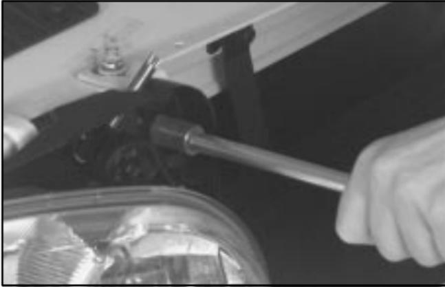
1. Remove the two bolts with a 10 mm socket.
